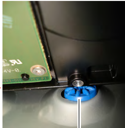
Align the hard drive screw hole with the blue rubber grommet.
