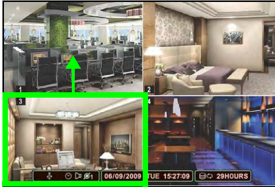
Press and hold inside channel 3 and drag your finger to move channel 3 to the channel 1 position.
