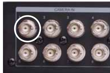
Figure 1.0 Connect BNC cameras to the system
