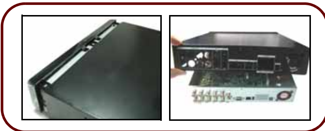
Slide the cover and lift away from housing
